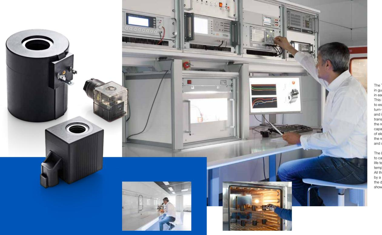
The Testing Laboratory plays a key role in guaranteeing the utmost quality in each stage of the production process. This includes the execution of tests to establish resistance strength, turn-to-turn insulation, insulation to ground, and inductance, with the ability to check transients, monitor temperatures, the residual magnetic value, the capacitance value and force-stroke graph of electric actuators as well as the response time of solenoid valves, and spectrographic analysis of materials.
